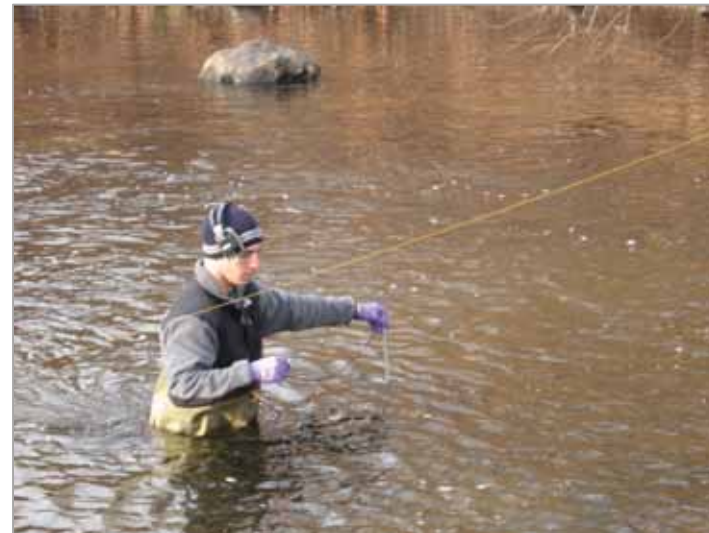
Measuring stream velocity of the Pomperaug River in Southbury (photo by Carol Haskins, Pomperaug River Watershed Coalition Outreach Director)
